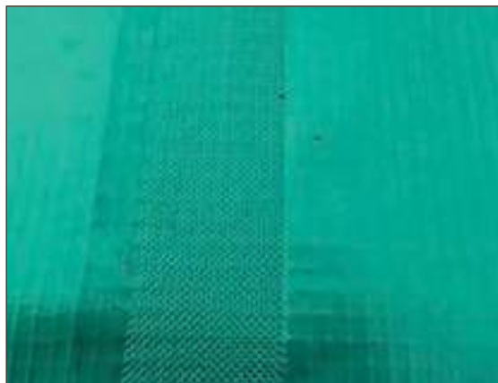
Figure A4.62 Wedge weld on an LDPE aluminium gas membrane, where the installer used metal nip rollers. This destroyed the top layer and probably the bottom layer, leaving aluminium exposed between the weaves. This failed dielectric testing along all joints (courtesy MEC Environmental Ltd)
