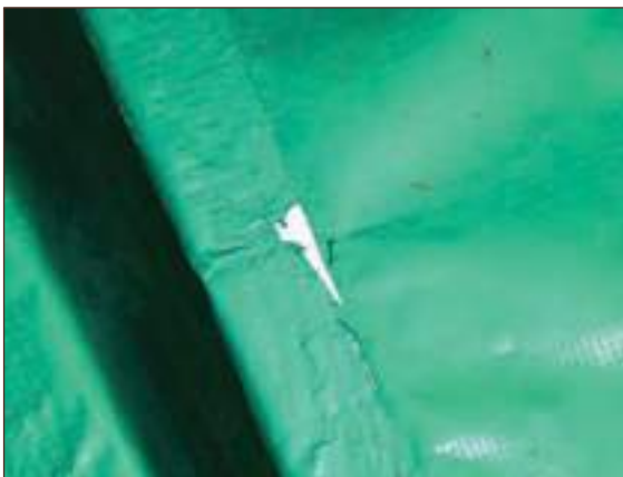
Figure A4.61 'Stripping' occurs on gas membranes that contain aluminium foil. The foil gets too hot under the outer layer of LDPE or PP and the top layer of the gas membrane sticks to the roller which strips it off, leaving the aluminium completely exposed (courtesy MEC Environmental Ltd)
