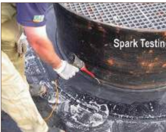
Figure A4.45 Spark testing (courtesy GSE Environmental)
